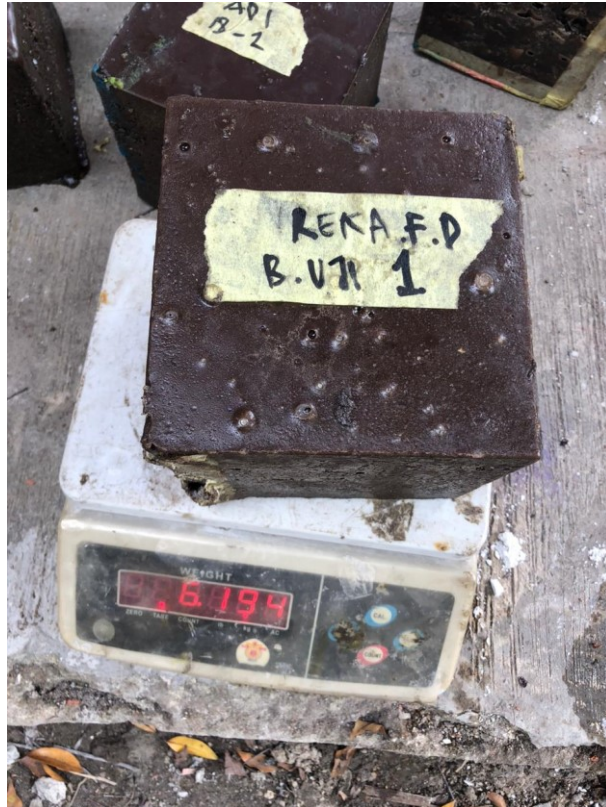
Gambar 4. 4 Benda Uji 1 Pasta Polimer 20%
