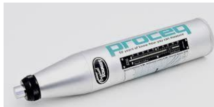
Gambar 2. 22 Alat Uji Hammer Test
